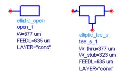
The open stub model (*open*) has one variable geometrical parameter, the width of the stub (W). There is only one relevant S-parameter, S<sub>11</sub>.
